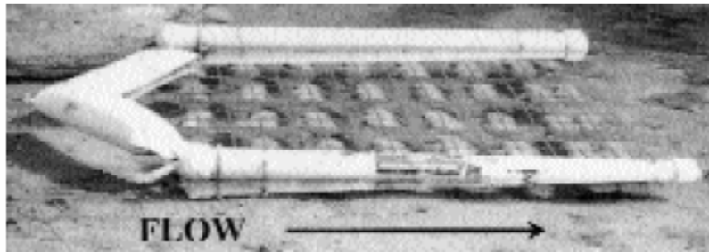
Figure 7. Diagrams of Matlock Periphytometer and photo showing Matlock Periphytometer treatment arrays. 11
